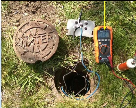
Measuring CP Effectiveness at Buffalo Box Test Station
