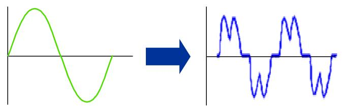
...but nonlinear devices distort voltage and current waveforms resulting in poor power quality on the distribution grid with further implications
