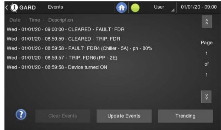
Figure 30: Momentary Feeder Fault Example
