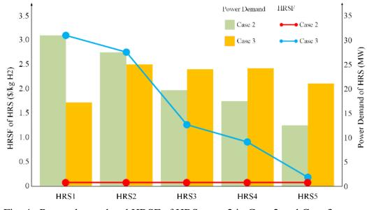
Fig. 4. Power demand and HRSF of HRSs at *t*=2 in Case 2 and Case 3.
