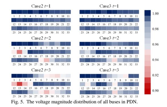
We can observe that Case 2 and Case 3 share the same voltage magnitude distribution in the first interval. This is because the UTN has a light traffic demand when t=1, no congestion occurs in both UTN and PDN. Thus, the voltage magnitudes are maintained within the normal range, and the HRSF is equal to 0 in Case 3 at t=1.
