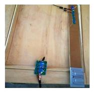
Power transfer over a latex paint conductive and carbon ESD spray conductive plane
